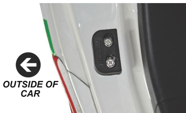
Figure 1 - how to position the polyurethane bush
