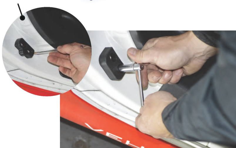
Figure 1 - how to position the polyurethane bush
